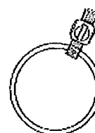
Corporation Stop Position
